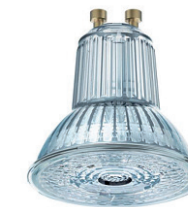
GU10 Art. L000000951 4,5W 2700K CRI90 350lm Ø 50mm H 54mm opal
