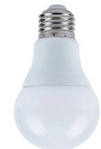
A60 Art. L000000952 8,8W 2700K CRI80 806lm Ø 60mm H 110mm opal
